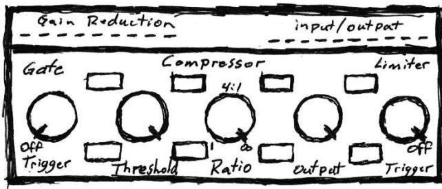
**Compression:** This begins to reduce the gain or strength of a signal once it crosses a settable threshold. This makes loud parts sound more similar to quieter parts and is used to make inputs of various strengths on an input sound more similar. There are a few settings controlled by knobs for this processor.
