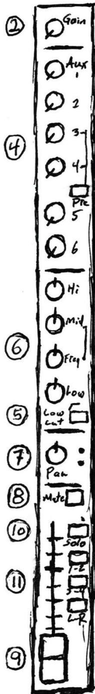
frequency you'd like to boost or cut. The “low” knob boosts or cuts frequencies of around 80Hz and lower.
